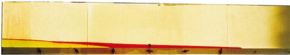
FIGURE 11. Long-time structure of a current produced from a source in which the low-viscosity upper layer was initially placed above the lower layer. In comparison with the flow shown in figure 6, there is a narrow strip of upper layer fluid which extends back to the source. This is a result of the viscous stress with the underlying layer.
